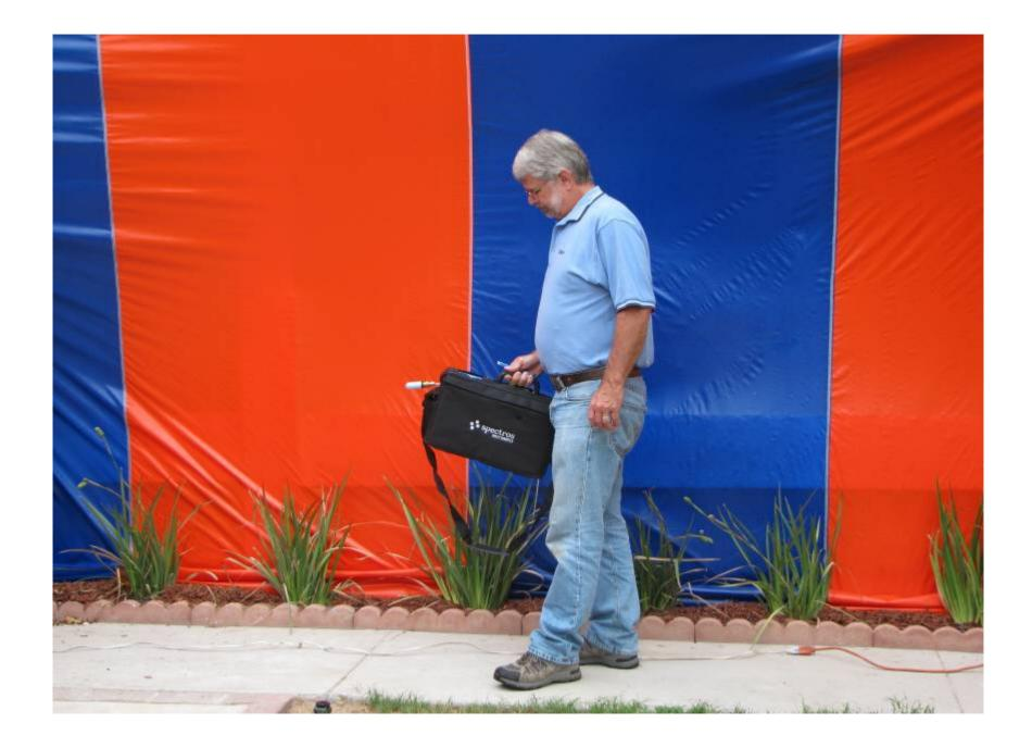
Interior fumigation concentrations were measured by drawing air samples through hoses placed at three locations indoors using the following validated testing procedures.
