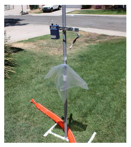
Fumigant concentration in each removed bag was measured using a sensitive gas monitor, the SF-ExplorIR, which can accurately measure sulfuryl fluoride concentrations to 1 part per million (1 ppm).
