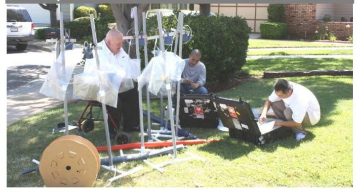
**Exterior fumigant** concentrations were continuously monitored at eight locations that were evenly spaced and close to the tarp. At each exterior sample location, a calibrated air pump attached to a stand continuously drew air into a gas-tight bag. At timed intervals, the air bags were removed from the pumps and immediately replaced with clean, empty, gas-tight bags attached to the pumps to continue with uninterrupted air sampling.
